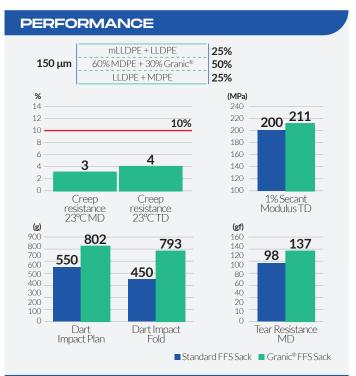
**Granic®** provides a specialised mineral masterbatch formulated with highly technical and ultrafine CaCO3, ensuring an excellent dispersion rate. When combined with highquality LLDPE, it significantly enhances the mechanical properties of the film, resulting in increased toughness and tear resistance.
