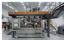
**Collin Twin–Screw Compounder Extruder** Fully customizable, especially suitable for high addition rates of mineral and functional fillers. Configured to handle sensitive materials, including biopolymers, natural fibers, and others.
